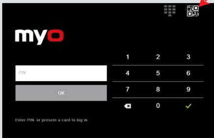
To print from your mobile phone/tablet, install application MyQ X, then just take a picture of the QR tag on the printer panel to automatically set up printing on your device.
